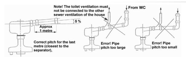
Use at least 110mm pipes between WC and Separator. For ventilation use 100mm (minimum) pipes.
