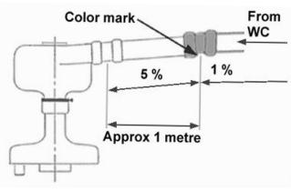
The ventilation should be installed between the WC and the Separator. The ventilation pipe should extend above the roof. If there is a large level difference between the WC-outlet and the Separator, then first install the horizontal pipe pitched at the specified angle, and then make the necessary level adjustment with the vertical pipe.
